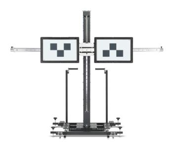
Q.DAS Pro | ADAS Calibration after wheel alignments
