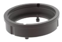
To be used in combination with light truck cone 1692502047 and spacer 1692502031. 40mm distance ring 1692502028 and spacer 1692502031 are mounted on the inside. Thel ight truck cone is used to lock the wheel from the outside. Spacer can be mounted either way, as long as it fits the inside rim shape.
